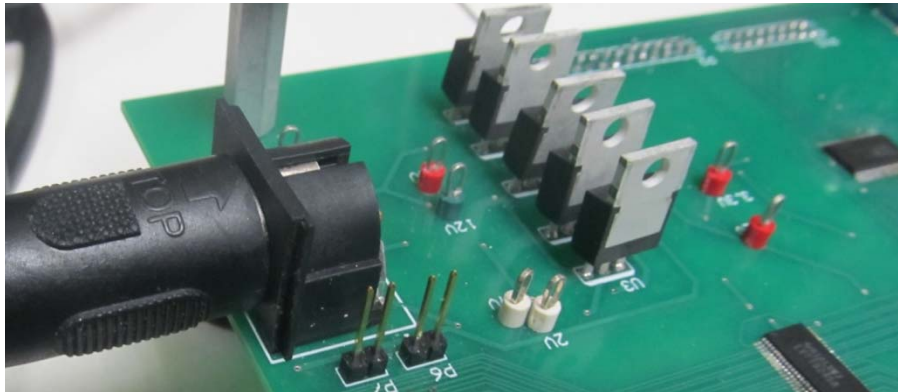
Power Supply Connected
